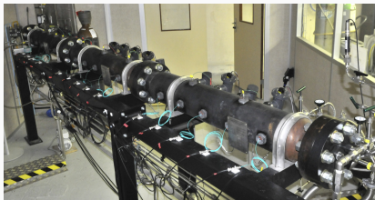
FIGURE 2 – Structures Submitted to an EXplosion of HYdrogen experiment
